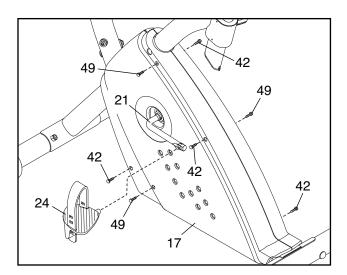
Next, locate the Reed Switch (43). Turn the Crank (21) until the Magnet (38) is aligned with the Reed Switch. Loosen, but do not remove, the indicated M4 x 16mm Screw (49). Slide the Reed Switch slightly closer to or away from the Magnet, and then retighten the Screw. Turn the Crank for a moment. Repeat until the console displays correct feedback. When the Reed Switch is correctly adjusted, reattach the left side shield and the left pedal.
